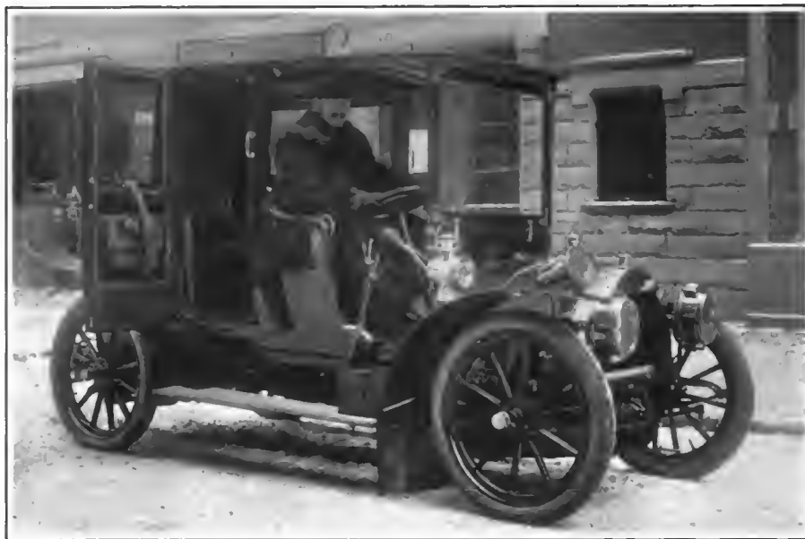
BELGIAN PIPE 15-20-HORSEPOWER CAR WITH CLOSED BODY FOR BAD WEATHER.
